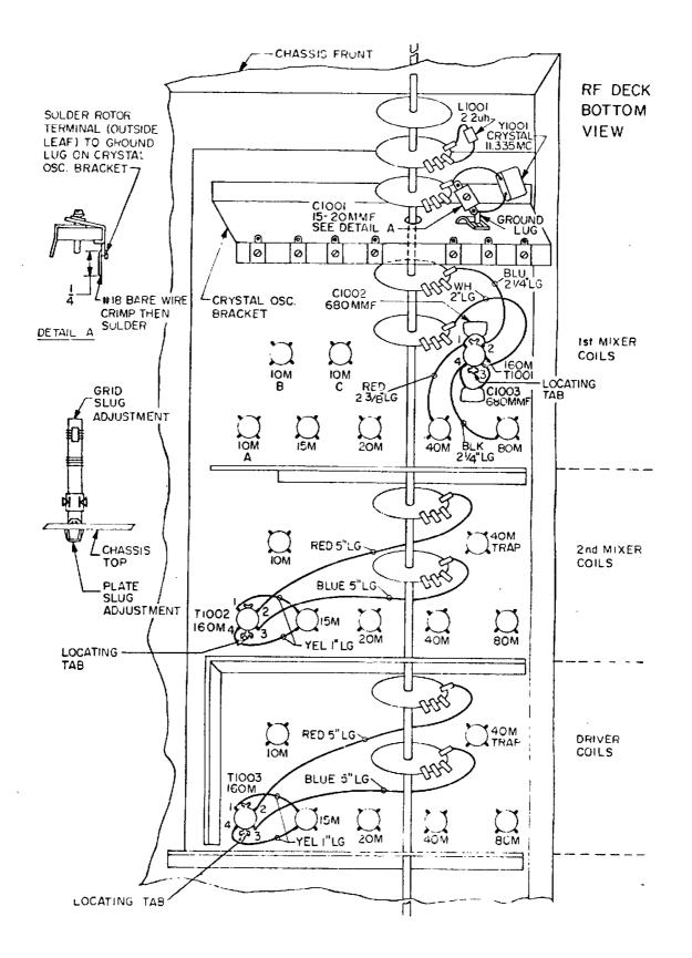
INSTALLATION DIAGRAM (160 METER KIT)
